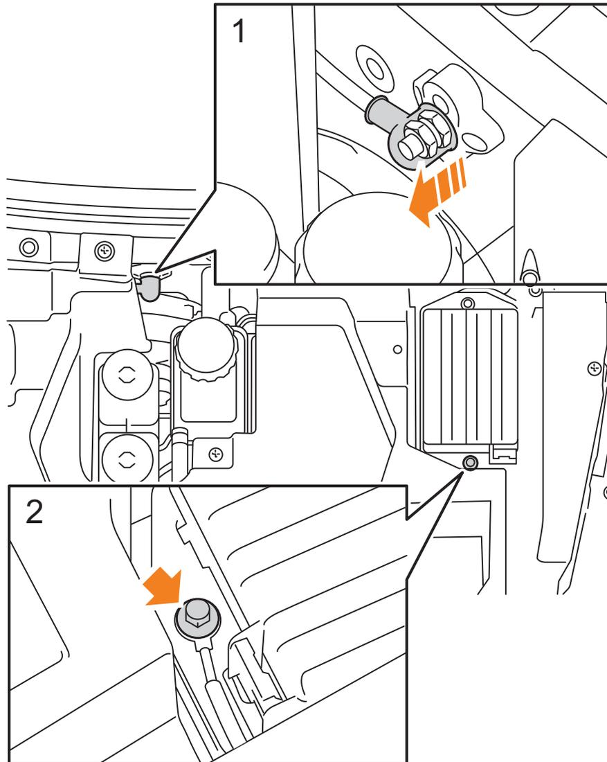
The vehicle's 12V battery terminals are located under the hood (see [“Hood”, page 19](#)) as follows:
