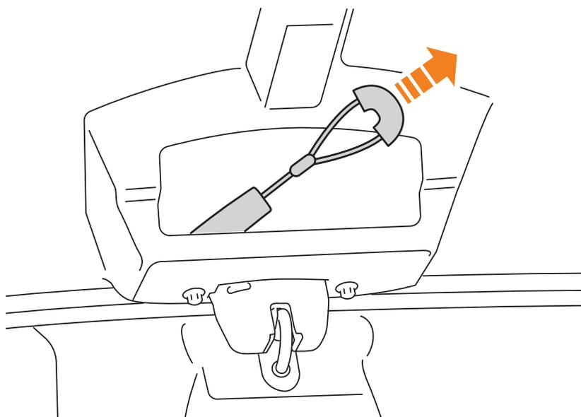
2. Pull the emergency release handle to unlatch the trunk.
