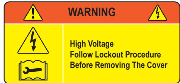
Illustrated above are examples of some of the high-voltage warning labels that can be found on high-voltage components within the vehicle. These labels are one way to quickly identify potential electrical hazards. For your safety, always follow all cautions and instructions on warning labels.
