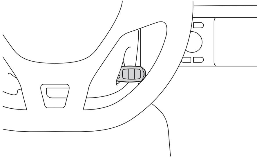
The key switch is a four-position switch that is located on the right of the steering column and is operated by inserting the key. The switch positions are as follows:
