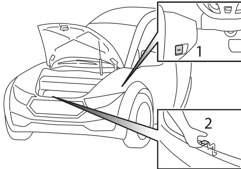
1. Pull the handle (1) located on the side panel under the lower left corner of the dashboard.
