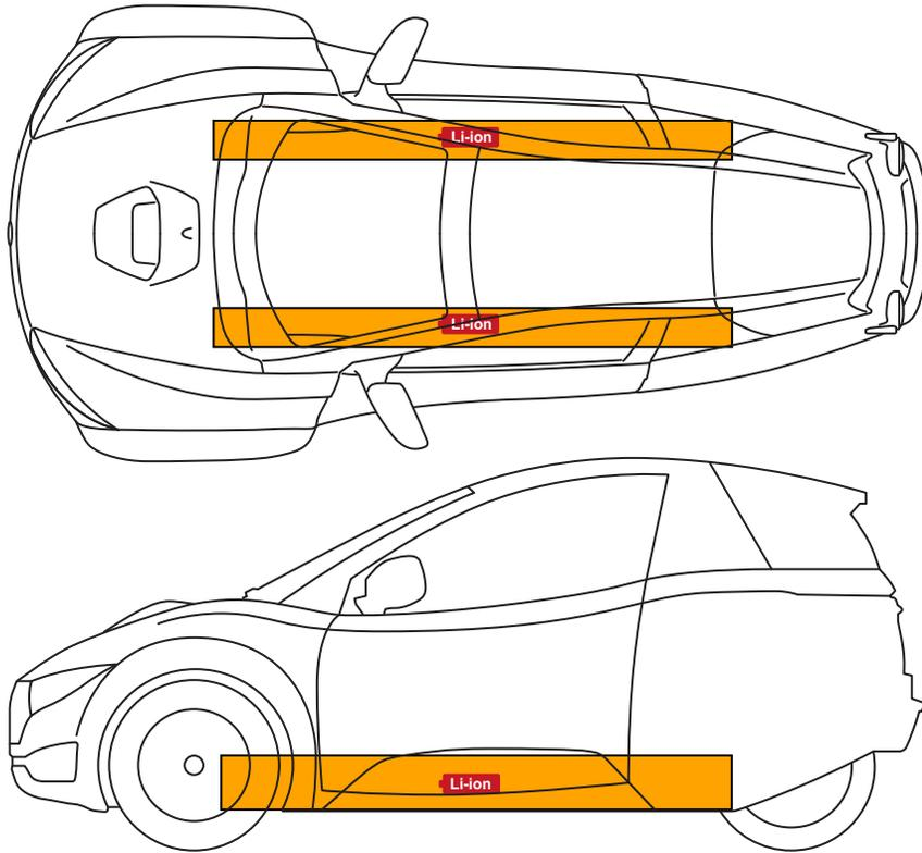
The 144V lithium-ion batteries are encased and mounted under the vehicle floor.
