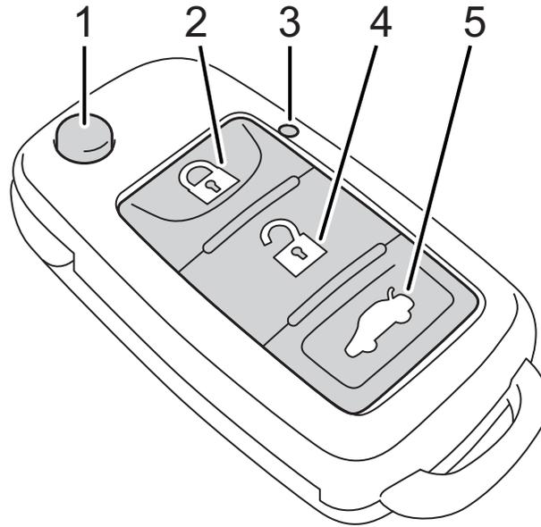
1. Key Release Button: Press to flip out the key blade.
