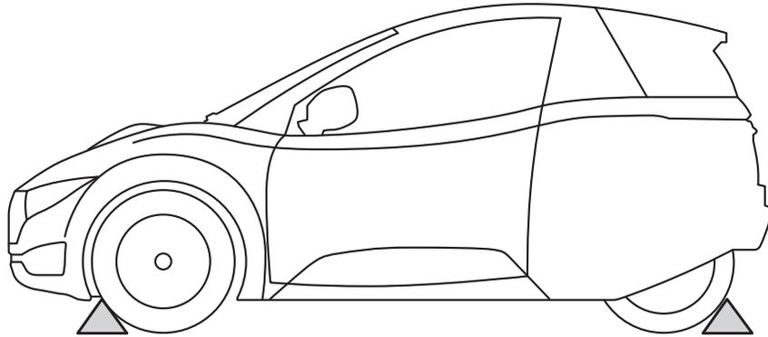
To help prevent the vehicle from moving, always chock all three wheels before attempting extraction procedures.
