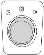
The current selection is illuminated on the dial, and is also indicated on the instrument cluster display.
