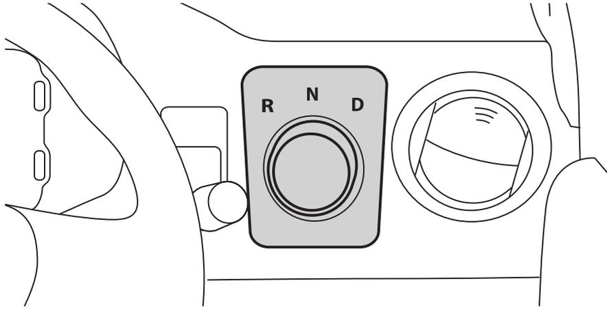
The Drive Mode Selector is a three-position dial on the dashboard. When the key switch is ON, the Drive Mode Selector can be used to set the desired direction of the vehicle:
