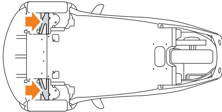
Use the two lower control arms (illustrated) as the hook/attaching points to secure the vehicle to a trailer.
