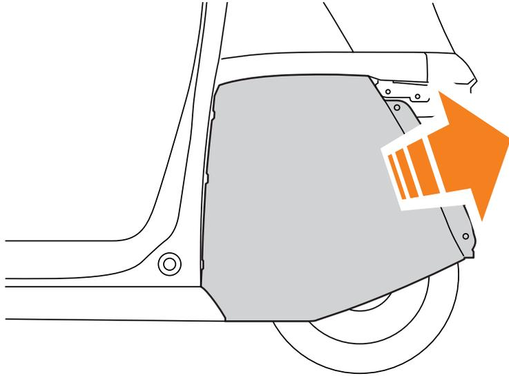
1. To access the high-voltage cables to be disconnected, use an insulated crowbar to pry off the left and right rear side covers.
