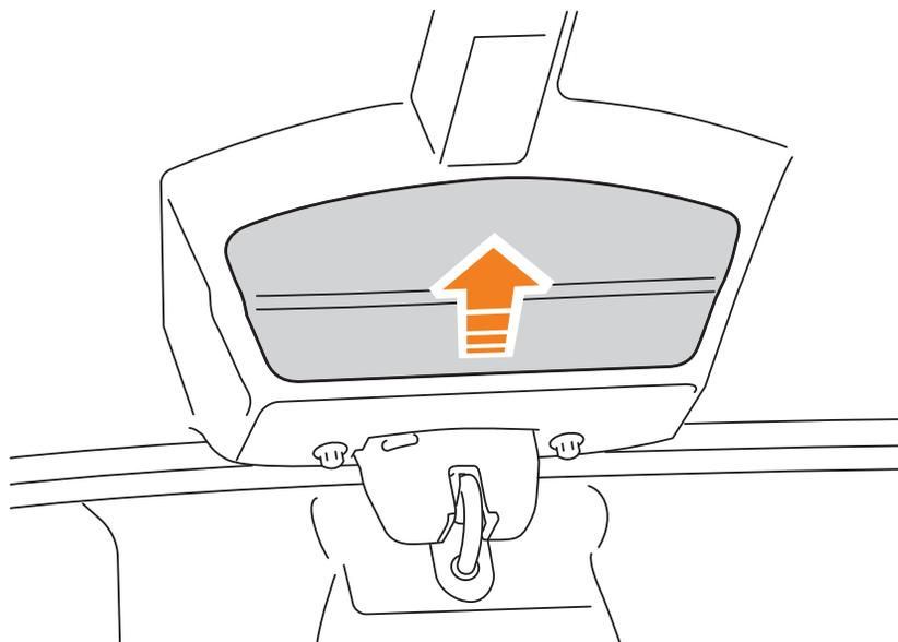
1. Remove the cover at the base of the trunk latch.
