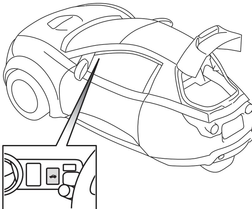
Pushing the trunk release button on the dashboard will open the trunk.
