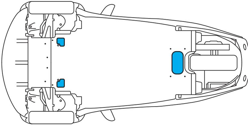
If the vehicle needs to be lifted, only use the illustrated lifting points to avoid breaching the high-voltage battery.
