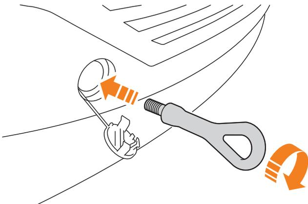
3. Insert the bolt fully into the recovery eye, then turn clockwise until it is tightly fastened.
