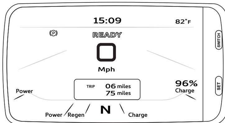
The READY indicator on the instrument cluster display signifies that the drive system is powered on and available.
