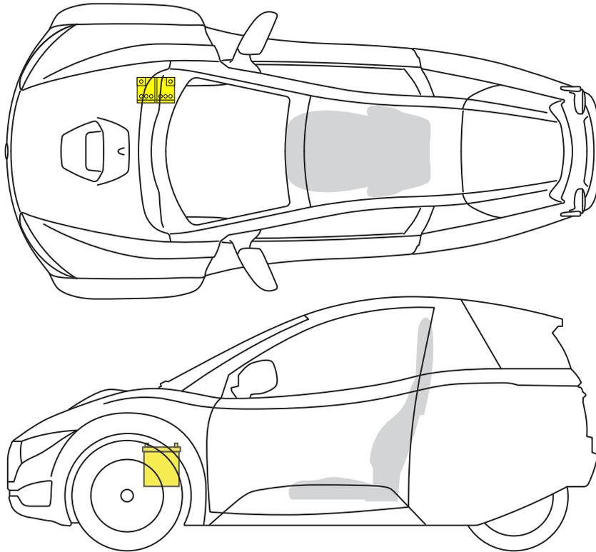
The 12V battery is located at the right front of the chassis, to the right of the accelerator pedal. This battery powers all of the standard low-voltage electronics in the vehicle. It also powers the high-voltage distribution box, which controls high-voltage current within the high-voltage components (e.g. drive motor, powertrain controller).
