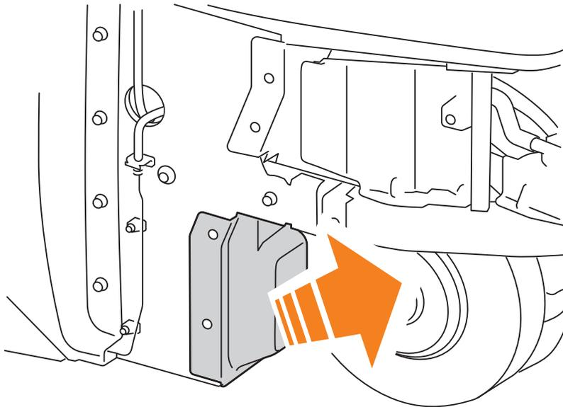
2. Use an insulated crowbar to pry off the left and right rear closeout panels.
