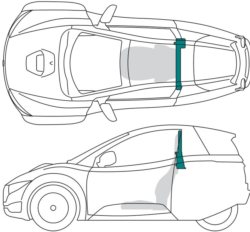
The roll bar and integrated belt anchor behind the seat can be more difficult to cut through, but it is safe to cut in this area if necessary.
