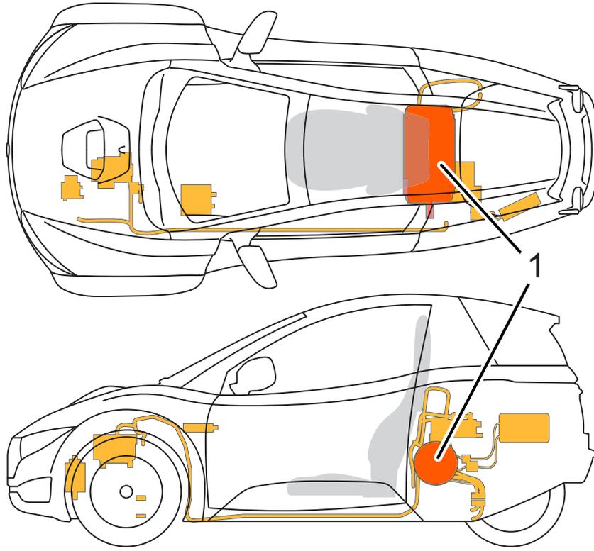
The drive motor (1) is located near the rear wheel of the vehicle. This component receives 3-phase alternating current (AC) and converts it into propelling energy (torque), used to power the wheels.
