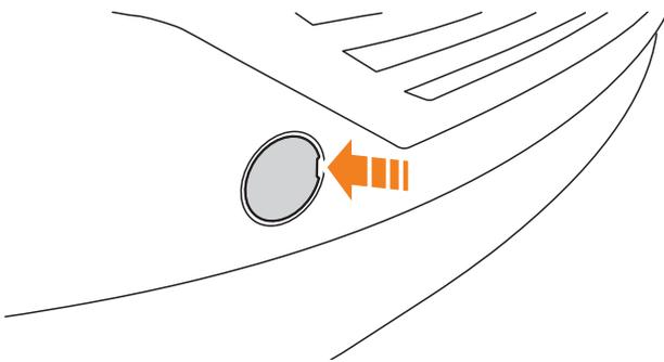
2. When facing the front of the vehicle, the recovery eye is located behind a cover to the right of the grill. To remove this cover, insert a flat-bladed tool (such as a screwdriver) into the slot along the edge, then gently pry up until it releases.
