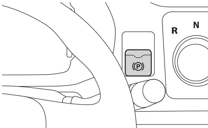
The EPB has both manual and automatic functions. It is manually controlled by a rocker switch on the dashboard, to the right of the steering wheel.
