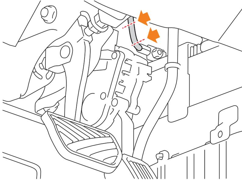
4. Locate and double-cut the 12V ground cable that runs from the 12V battery negative to the steering column bracket. Be sure to cut out a section of cable that is wide enough to prevent the cut ends from accidentally touching and completing the electrical circuit.
