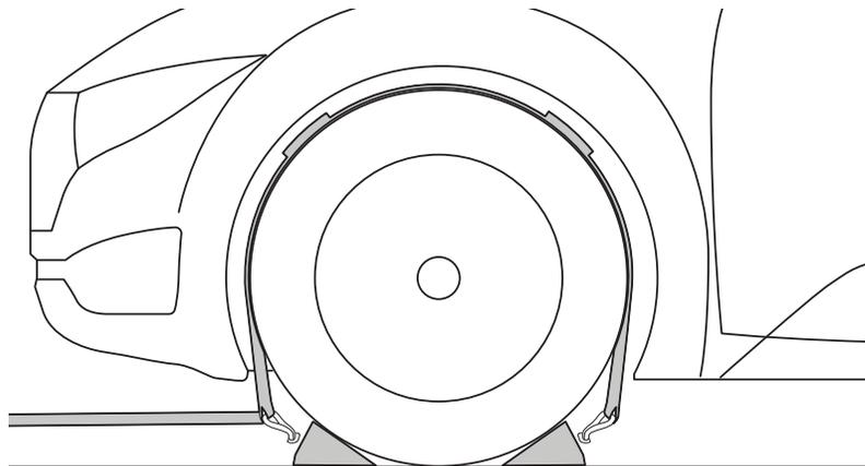
8. Use tire wheel straps or loop straps (illustrated) to secure the vehicle to the trailer or flatbed transporter.
