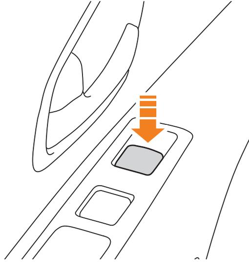
The power window switches are located on both of the side door panels, and each switch controls its own window. To operate a window:
