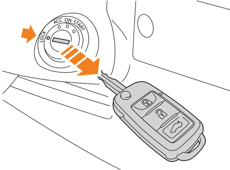
3. Turn the key switch to the OFF position and remove the key. See [“Using the Key Switch”, page 24](#)
