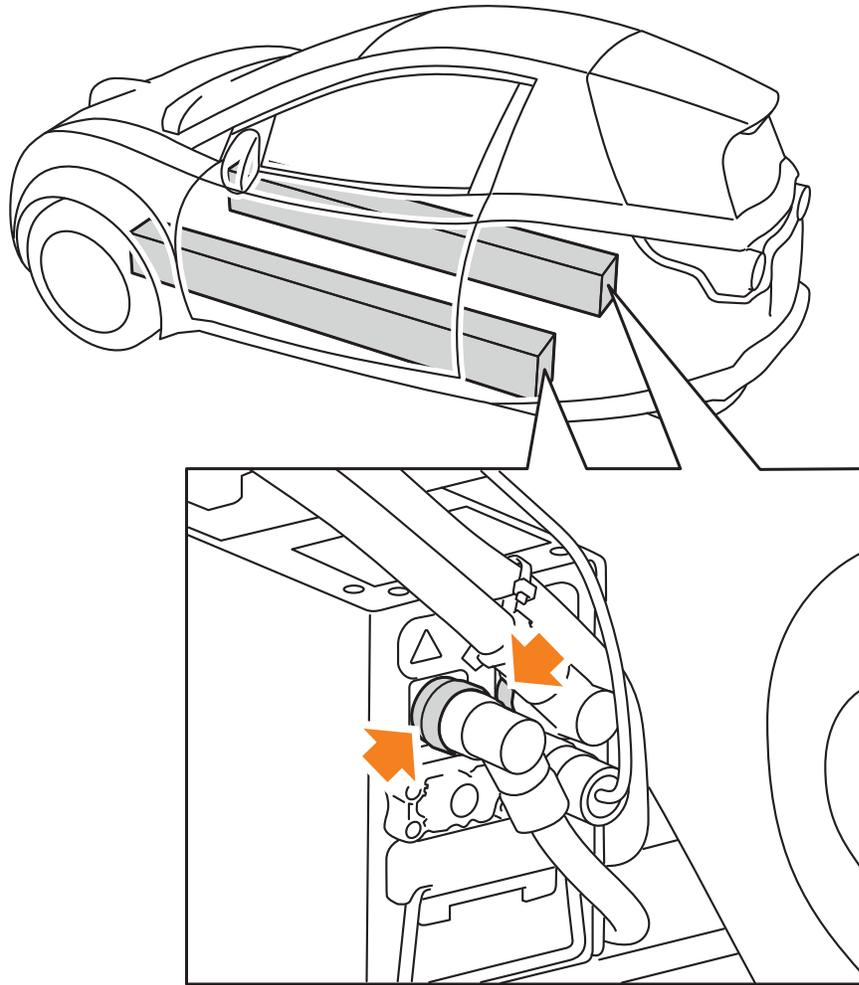
3. Rotate the locking collar and disconnect B- high-voltage cables from both the left and right battery assemblies.
