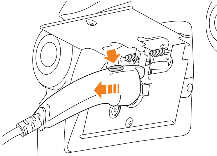
1. Press the button on the charge cable connector to release the locking clip.
